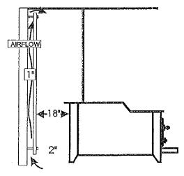
Stove & pipe may be placed within 18" of a wall or combustibles if protected. Protection consists of a panel of non-combustible material spaced 1" from the wall & 2" above the floor. The spacing allows a flow of cool air to reduce the heating of the wall or combustibles.
