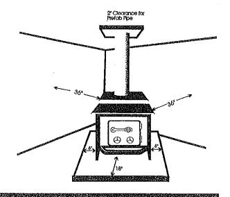
A freestanding woodstove requires 36" of clearance from the stove and stove pipe to combustibles on all sides. Also required is floor protection that extends 6" on the non loading sides and 18" on the loading side of the stove.
