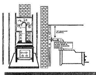
Where the stove pipe enters a thimble, the thimble must be surrounded by at least 18 inches of solid masonry
